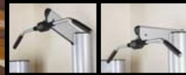
The high pulley adjusts from 6'6" to 6'11" to accommodate various ceiling heights and physical characteristics of the primary users.
